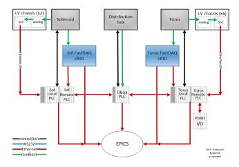
FIG. 3. Proposed Torus and Solenoid control and monitoring system. Version one of the upgrade uses special software developed for communication between the LV chassis and the PLCs. The EtherNet/ IP real time protocol software indicated by the label on the red line between the LV chassis and the Torus/Sol PLCs will not be needed. Upgrade version two does use the EtherNet/IP real time protocol software. Both versions of the upgrade eliminate the Torus/Sol LV cRIO.
