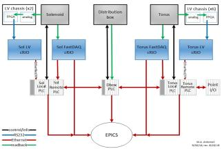
FIG. 1. Torus and Solenoid control and monitoring systems.
