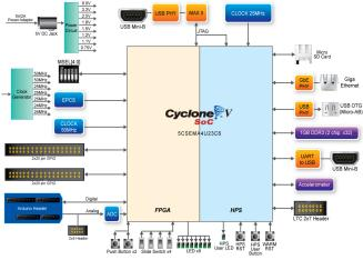
FIG. 2. DEO-Nano-SoC block diagram [3].
